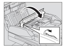
5 Raise the guide plate under the transport guide, and then release the original jammed under the guide plate.
